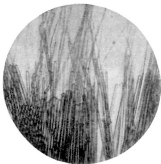
Fig. 6.—Filaments of 3-16 \omega -ester spun from chloroform solution showing transparent fibers produced by cold drawing ( \times 15 ).
